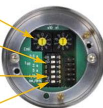
"plus" types can alternatively switched in online mode to enable the communication via serial interface and software *InfraWin* (in scope of delivery) on a PC. This allows additional setting options as well as the graphical temperature display combined with subsequent analysis of the measurement values.
