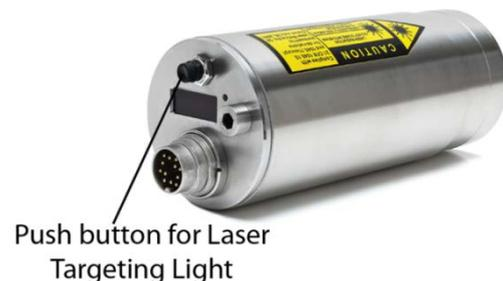
To prevent damage to the laser, the targeting light is also switched off automatically if the internal temperature of the pyrometer exceeds 61 °C. It can only be used again once the temperature falls below 61 °C.
