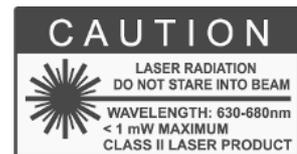
Never look directly into the laser beam. The beam and spot can be watched safely from side. Also, make sure that the beam will not be reflected into eyes of people by mirrors or shiny surfaces.
