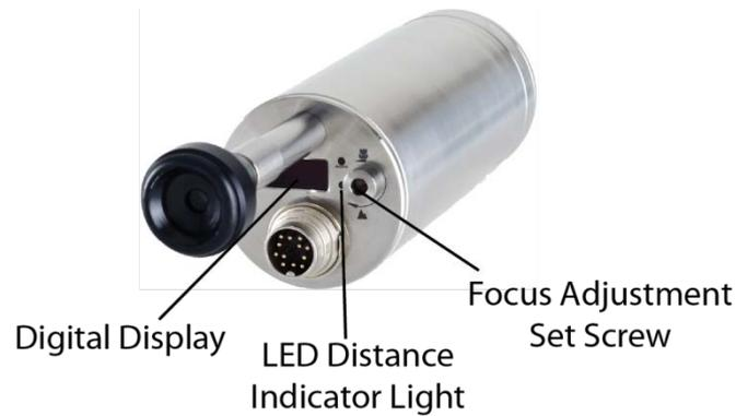
The LED Distance Indicator Light (labeled mm) will turn red and the approximate focused measuring distance in mm will automatically be shown on the Digital Display for a few seconds after making an adjustment using the Focus Adjustment Set Screw.
