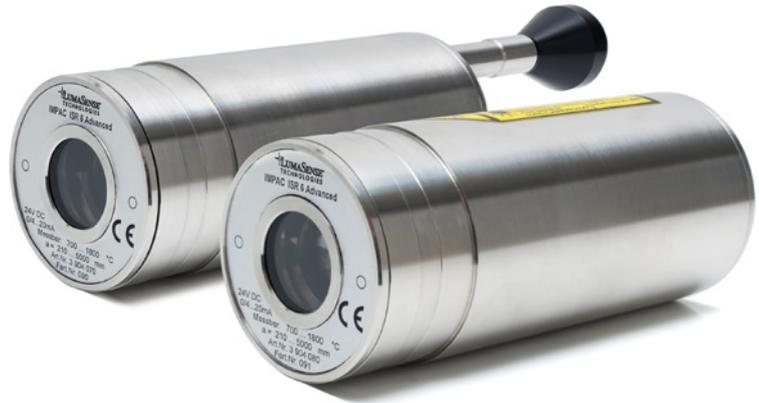
The ISR 6 Advanced pyrometer is a digital, compact and fast 2-color pyrometer for non-contact temperature measurement. The pyrometer measures in the 2-color method (ratio method) in which two adjacent wavelengths are used for the temperature determination.
